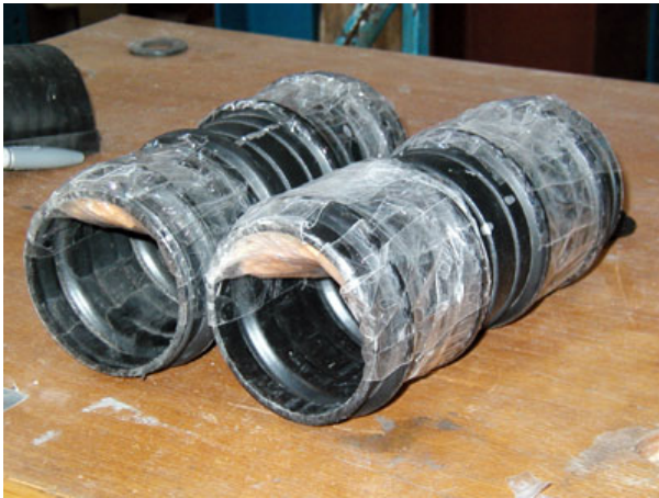
(a) Sponge attached to sections of duct
