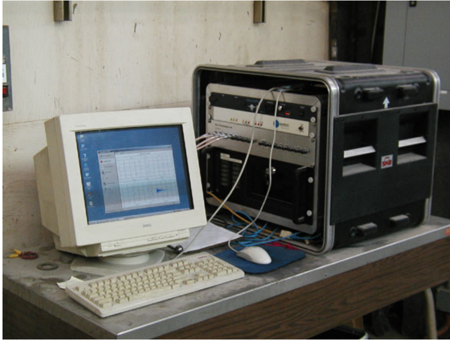
Figure 4.4 Watch Dog-PS6 (SoundPrint™) Hardware
