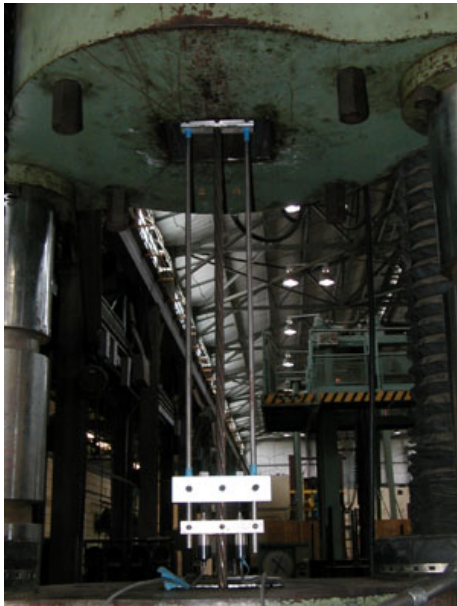
(a) Apparatus for supporting displacement transducer
