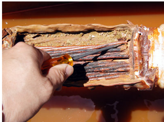
(h) Visual observation of broken wire
