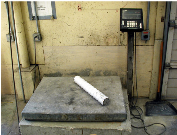
Figure 6.2 Portion of Test Specimens used to Determine Weight per Unit Length
