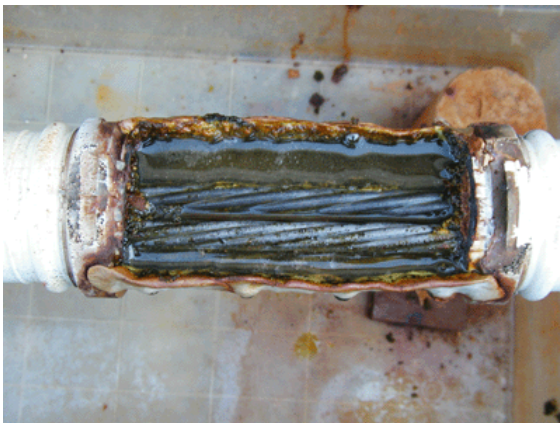
(g) Void filled with acid
